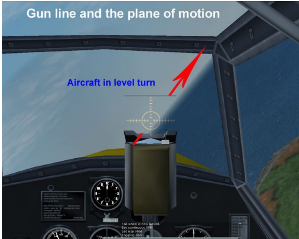
Figure 21 – Gun line and plane of motion
